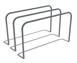
The construction consists of three curved bars that are placed parallel. The distance between the inside surfaces of bars is 500 mm. The horizontal surface of bars is 1650 mm in length. Bars are symmetrically curved at the angle of 90 degrees and create the construction at the height of 1200 mm (1300 mm optional height is possible) from the foundations. Weight 78 kg.
