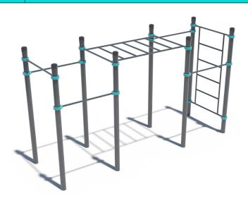
The complex consists of eight vertical columns, five crossbars 1200 mm in length, Swedish wall and a classic monkey bar. Optionally, two 1200 mm crossbars can be re-designed to be 1758 mm in length. Height of the Swedish wall - 2073 mm, width - 1200 mm. The distance between the crossbars of the Swedish wall - 407 mm. The length of monkey bars is 1900 mm. The distance between the crossbars of the monkey bar is 311 mm. Construction is secured together with siluminium clamps. Weight 376.4 kg.
