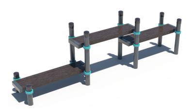
The construction consists of eight vertical columns of different height, six crossbars 490 mm in length, supporting three sets of composite material benches. The beam length of each bench is 1500 mm. All elements of the construction are secured together with siluminium clamps at the height that corresponds to the wishes of the Client. Weight- 248,4 kg.
