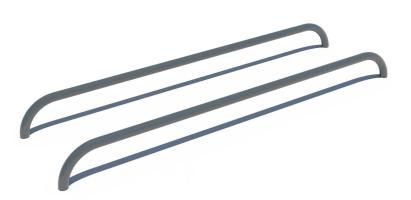
The construction consists of two curved bars that are placed parallel. The distance between the inside surfaces of the bars is 500 mm. The upper horizontal surface of the bars is 1650 mm long. Bars are symmetrically curved at the angle of 90 degrees and create the construction at the height of 300 mm from the foundations. Weight 32 kg.
