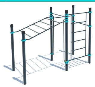
The complex consists of six vertical columns of different height, an inclined monkey bar section, a Swedish wall section, two crossbars 1200 mm in length and two climb-down bars 1932 mm in height. The length of the inclined monkey bar - 1790 mm. The distance between the crossbars of the inclined monkey bar is 350 mm. The difference between the lowest and highest point of the inclined monkey bar is 466.3 mm. The structure is secured together with siluminium clamps. Weight - 286.10 kg.
