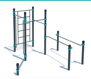
The complex consists of eight vertical columns of different height, four crossbars 1200 mm in length, a Swedish wall section, two climb-down bars 1932 mm in height and two parallel bars 1932 mm in length. The distance between the inside surfaces of the parallel bars is 550 mm. The height of the Swedish wall is 2073 mm, width - 1200 mm. The distance between the crossbars of the Swedish wall - 407 mm. The structure is secured together with siluminium clamps. Weight - 284.70 kg.
