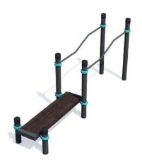
The complex consists of six vertical columns of different height, two crossbars 490 mm in length, multi-level parallel bars 1790 mm in length and a composite material bench. The distance between the multi-level parallel bars is 598 mm. The difference between the lowest and highest point of the multi-level parallel bars is 300 mm. The structure is secured together with siluminium clamps. Weight - 152.80 kg.
