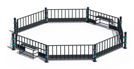
The structure consists of eight vertical columns 900 mm in height and eight sections with vertical crossbars. Height of each section is 800 mm, length - 2381 mm. The structure is secured together using siluminium clamps.
